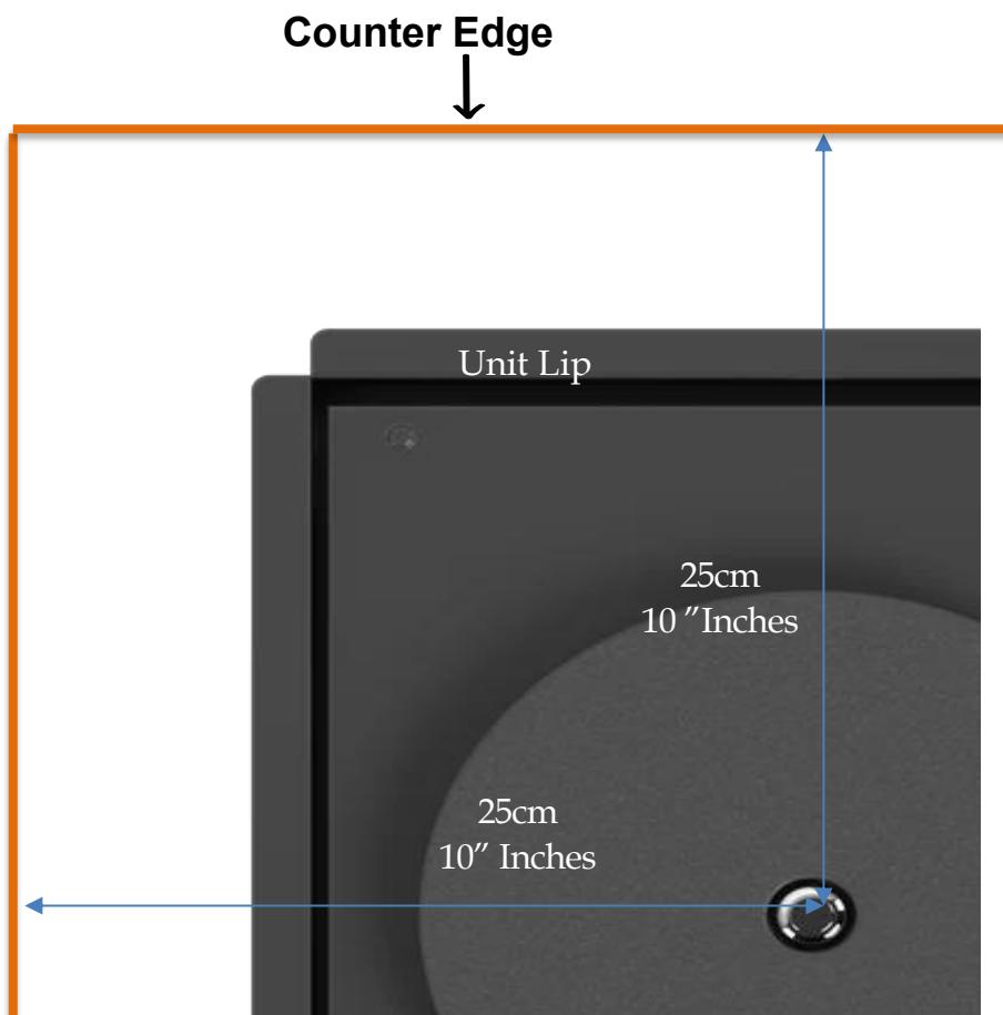
*Invisacook can only be used with a minimum countertop thickness of 12mm (1.2cm) (1/2") and Max thickness of 20mm (2cm) (3/4") Countertops from tested and approved brands*
