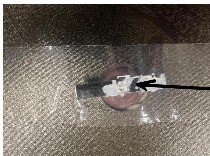
All Burners are equipped with a Dural Sensor as seen in the image to the right. Upon this Sensor is a White Thermo Gel, which must remain on when installed. Only remove the clear plastic tape before installation.
