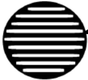
Vents are on the underside of the units, which allows the fans to properly vent and cool down the system from below, which look like this image. 2 Burners will have 1 vent, 3 and 4 Burners will have 2 vents and 5 Burner will have 3 vents that must not be obstructed.
